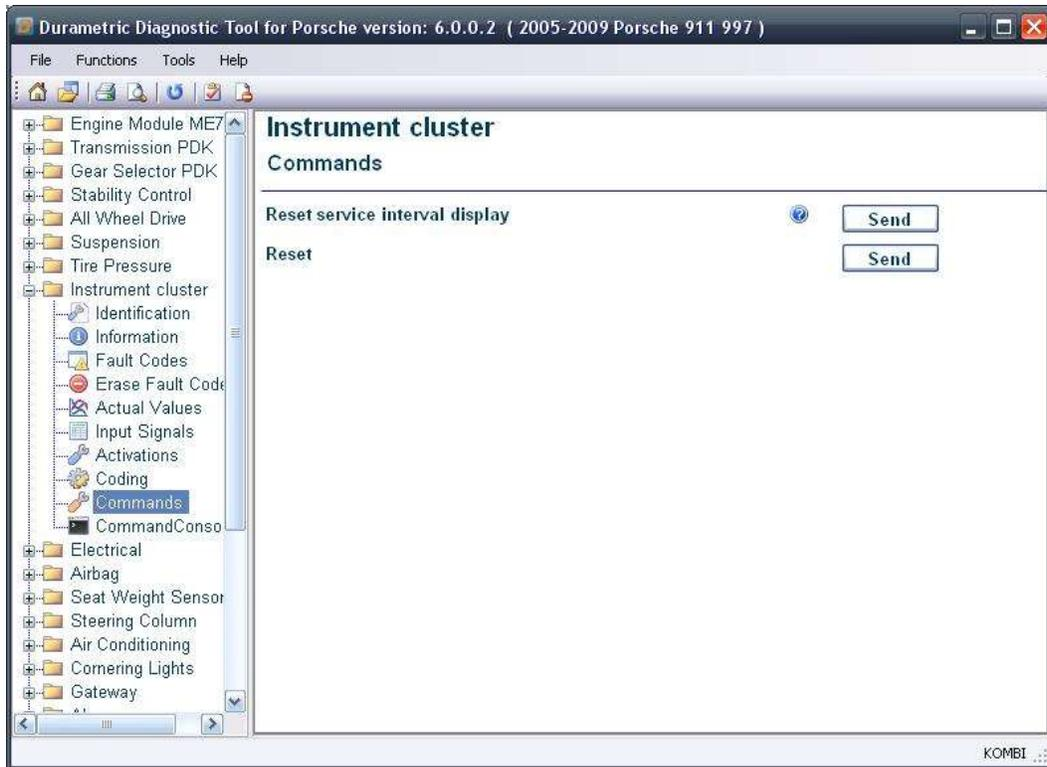
Find service interval resets under the *Commands* option of the instrument cluster
